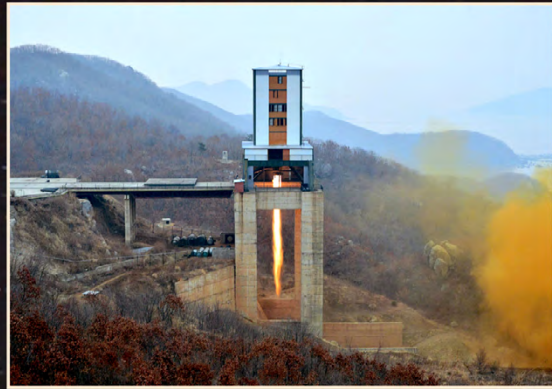
March 18, 2017 Static firing test of a newly-developed high-thrust motor
