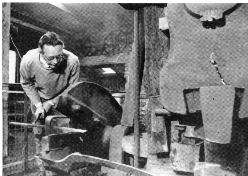
Below, Mr R. A. Barron at work on the power shears. The steeling hammer with inter-changeable bit inserted between chocks can be seen in close-up on the right.
