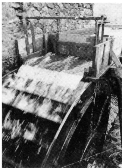
The 12 ft. overshot water-wheel which powers the hammers, shears and drop stamps in the forge area (left). The flow of water from the reconstructed laundry is controlled by a lever-operated hatch.
