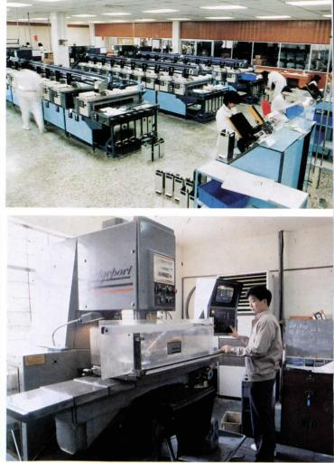
The Zhuhai Xinghua Component Factory produces printed circuit plates and name plates with computerized electrolytic corrosion spark machines imported from Japan and exports part of its output.
