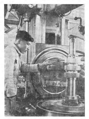
Eighteen-year-old Tung Ping-fang, after one year's apprenticeship, can operate this gear hobbing machine made in Czechoslovakia
