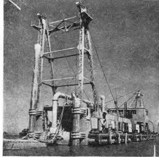
Only 3,000-ton vessels could reach this area before modern suction dredgers like the one shown deepened the channel for 10,000-ton ships
