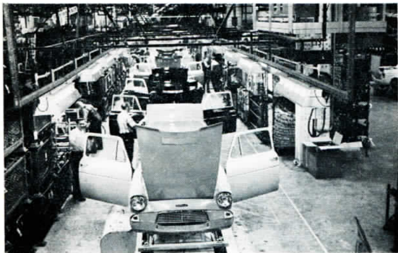
A typical line where speed-up occurs on the last in first out principle.
