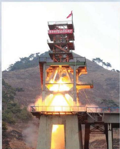
탄도로케트 대기권재돌입환경모의시험 Re-entry simulation test of ballistic rocket
