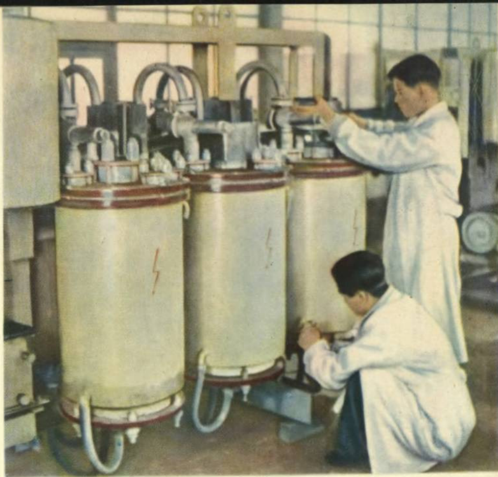
Assembling of a mercury rectifier at the Pyongyang Electric Appliances Factory
