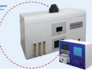
The surface alloy device alloys metal surface through micro electric discharge. Through electric spark discharge between the alloy electrode (positive) and the processed metal product (negative), the device covers the product with alloy coating of wear resistance.
