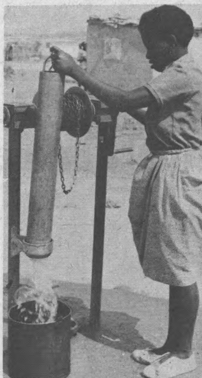
Bucket pump — improved version of the ordinary well
