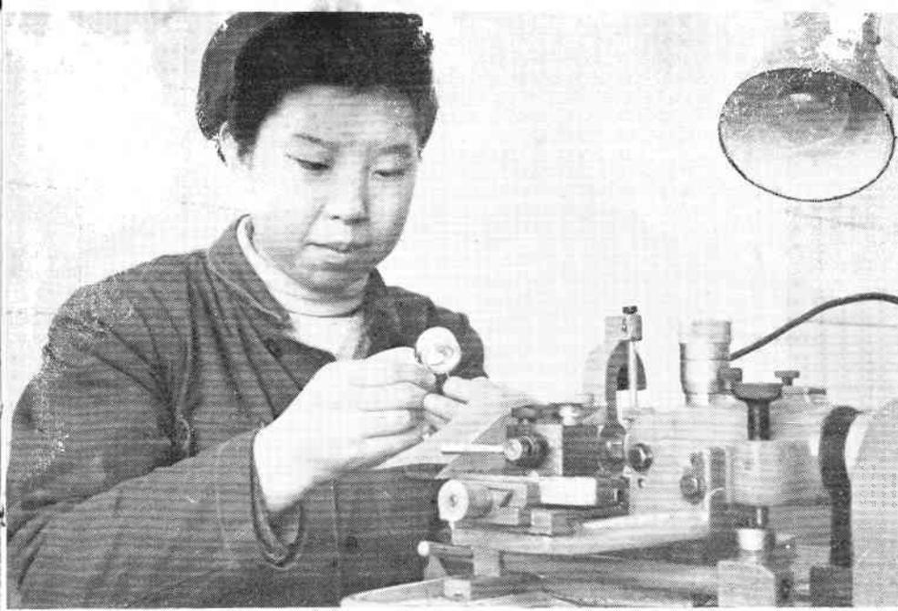
Feng Shen checks the new 25 mm. drill-heads she made in a Harbin instrument works. They are used in making precision instruments, watches, clocks, etc.
