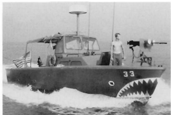
This Landing Craft Personnel (Large) MK II (LCPL MK II), based in Cat Lo, cruises in Vung Tau harbor, the entrance to the main shipping channel to Saigon. The sharkmouth on the bow is an unusual marking for a small Navy craft. The aft .50 caliber machine gun has not been fitted. (US Navy)
