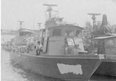
During this period more and more American brown water assets were turned over to the Vietnamese. Among these were Mark II Swift boats seen just after their turnover. One of the main distinguishing features between the Mark I and II was the ralling toward the bow and the port-hole shapes along the superstructure. (O'Mara)
