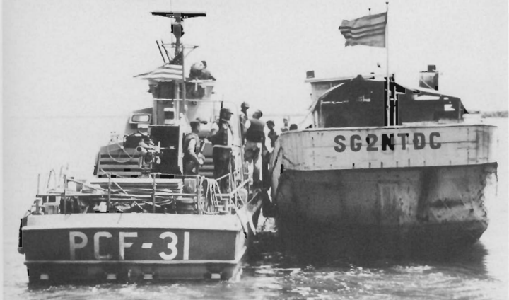
(Above) For close-in work Patrol Craft, Coastal (Fast) (PCFs), nicknamed 'Swift boats', with their shallow draft were ideal. These boats, modified from crew boats used to serve commercial oil rigs, carried a twin machine gun turret atop the cabin and mortar/machine gun combination aft. (US Navy)
