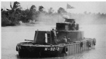
Fire support was an important part of the riverine force's job during an operation. This Monitor fires its 40mm cannon on enemy positions during operations in the Delta. Note how the crew take advantage of the turret and superstructure for protection while observing the effect of the fire. (US Navy)
