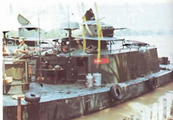
An Assault Support Patrol Boat (ASPB) moored along a shoreline during a break in operations. Note the use of heavy mesh screening around the forward turret to detonate RPGs before they hit the turret. (Benedetti)
