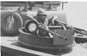
The PBR carried heavy fire power for such a small boat. The forward turret carried a pair of .50 caliber machine guns and a co-axially mounted searchlight. Late in the war a 20mm cannon was fitted in the turret, replacing one of the fifties and was fired alongside the remaining fifty.
