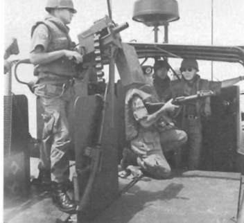
During a visit to Vietnam Secretary of the Navy, Paul R. Ignatius, inspected the armament of a PBR. In the stern a variety of weapons could be mounted, in place of the usual fifty. This boat carries a rapid fire 40mm grenade launcher and a single M-60 machine gun on a starboard side mount behind the cockpit. An M-16 rifle and M-79 grenade launcher are carried as personal weapons by the crew. In addition, another .50 caliber machinegun is also mounted further aft. The crewmember demonstrating the grenade launcher is wearing the famed Black beret. (US Navy)
