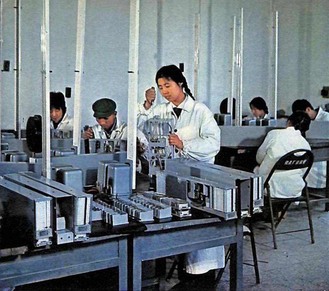
Assembling IC electronic controls and instruments at the Lanchow Oil Refinery.
