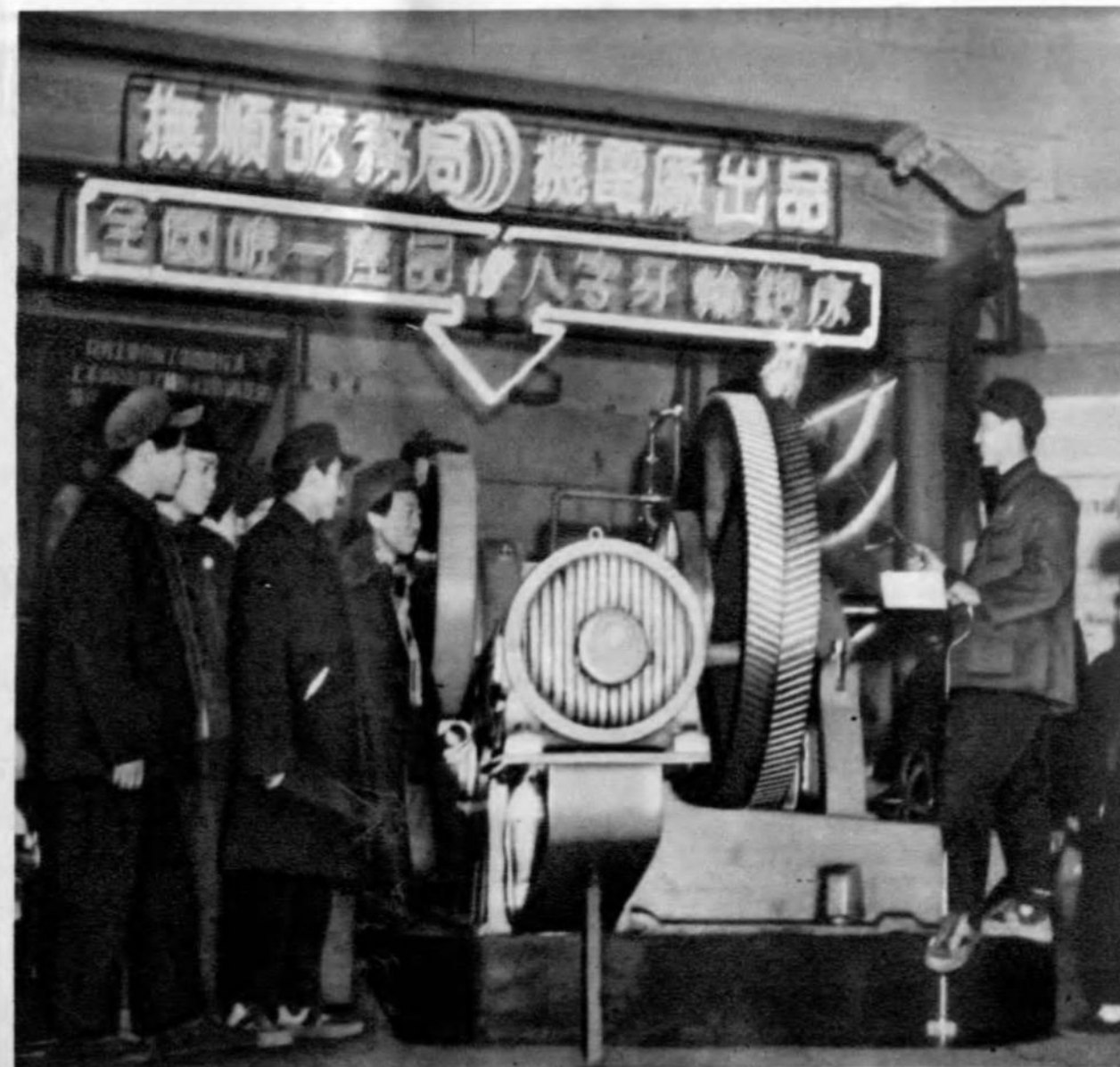
A bevel-gear planer made of nodular cast iron, displayed at the Northeast Trade Exhibition
