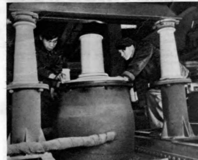
Workers of the Mukden Metallurgical Works maintain the efficiency of the electric dust collectors by constant overhauling. Smoke and dust contain many valuable materials which can be collected and refined
