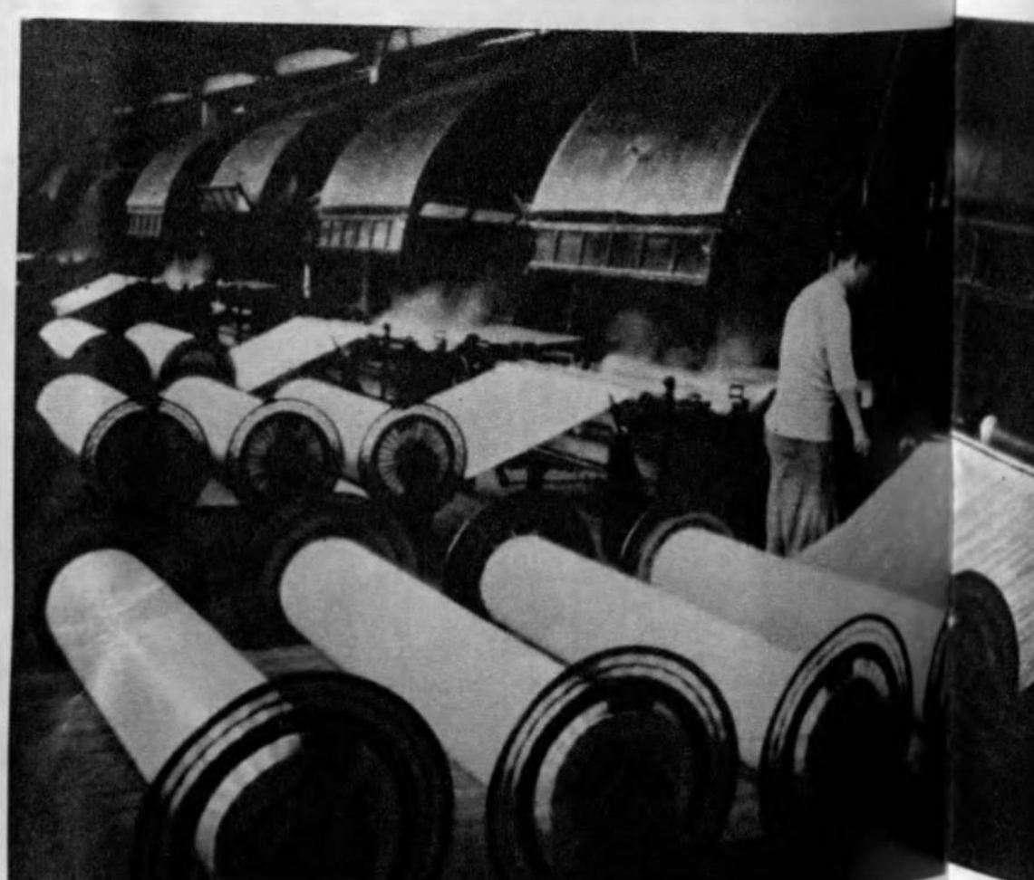
SIZING —the warp beams are taken into the sizing room where the yarn is sized and dried. The main substances used in sizing are flour and starch. The object of sizing is to increase the strength of the yarn to enable it to bear the strain of weaving
