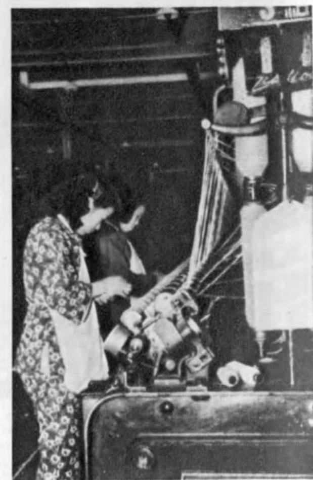
FINE SPINNING —fine yarn is produced on a ring frame
