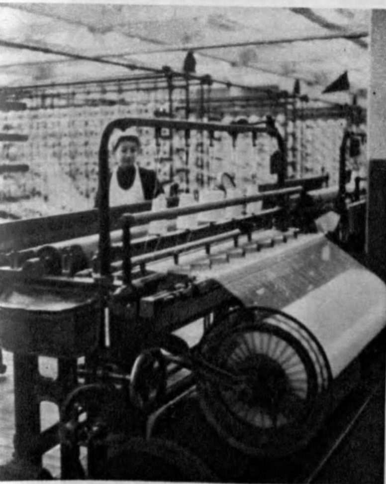
WARPING —the yarn is wound on a warp beam
