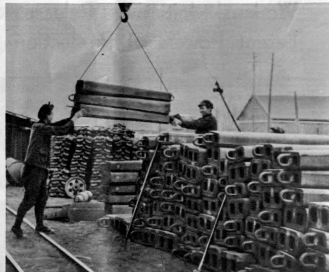
Nodular iron castings produced by the engineering department of the Fushun Colliery
