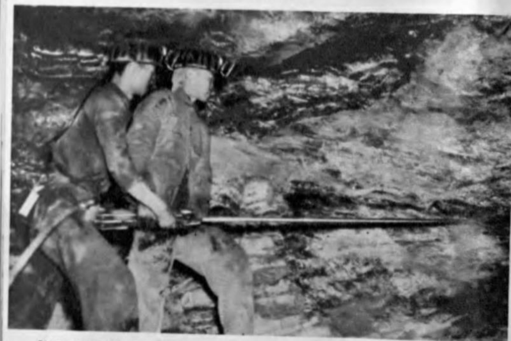
New record in coal cutting —A team of miners in the State-owned Pingsiang Colliery in Kiangsi Province, composed of six drillers and timberers and four truck drivers, have created a new national record in coal cutting. Above: Drillers Hsieh Fu and Wang Chao-yun prepare holes for the insertion of charges
