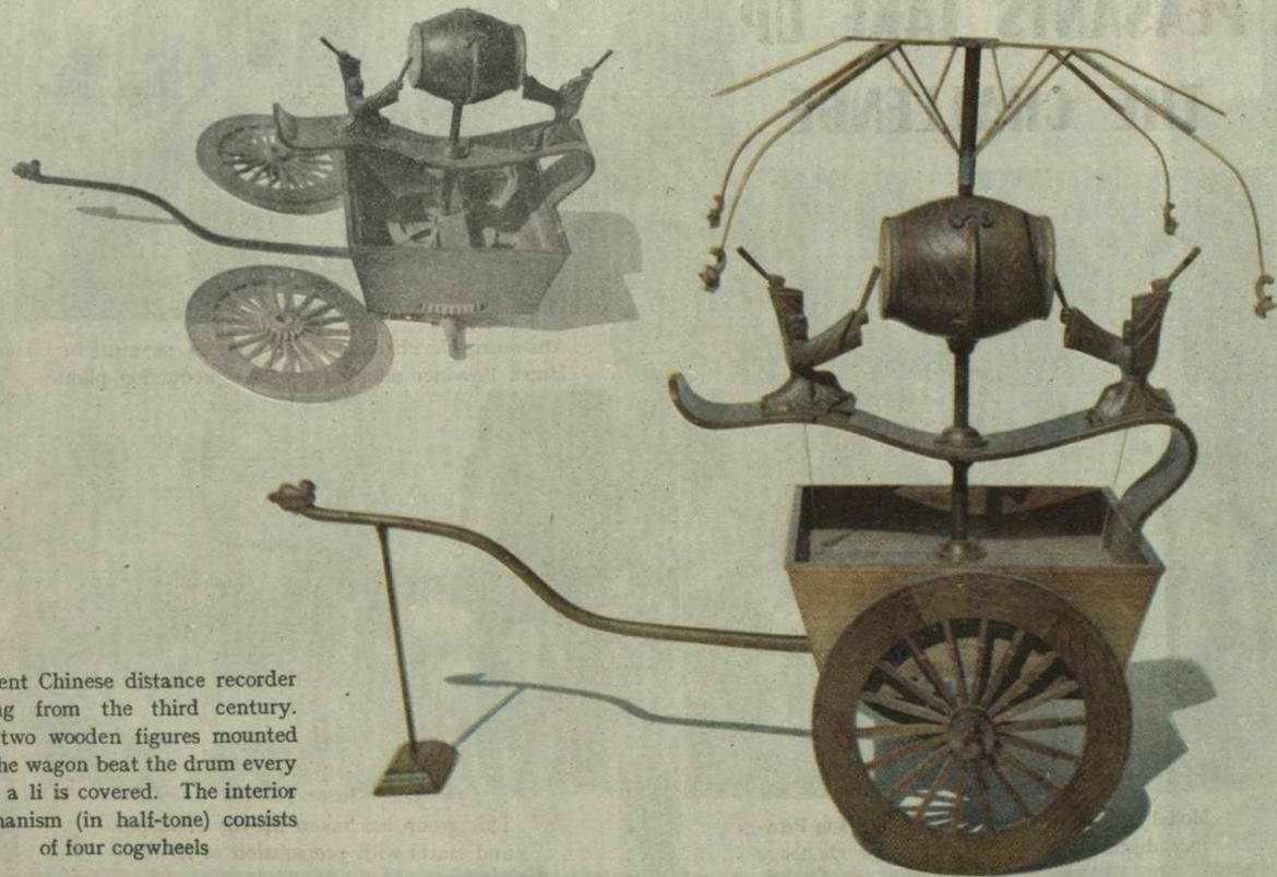
Ancient Chinese distance recorder dating from the third century. The two wooden figures mounted on the wagon beat the drum every time a li is covered. The interior mechanism (in half-tone) consists of four cogwheels
